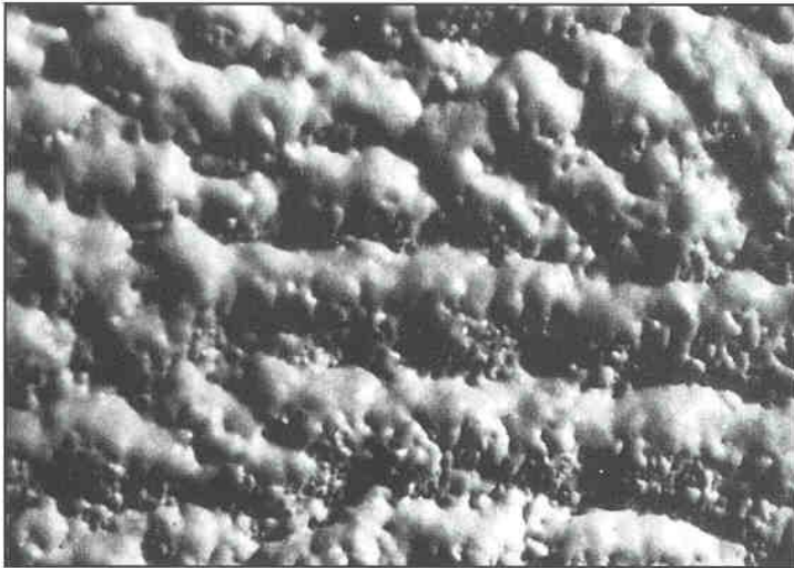
Photo 4 Polyurethane Foam Texture Rippling – Verge of Popcorn
