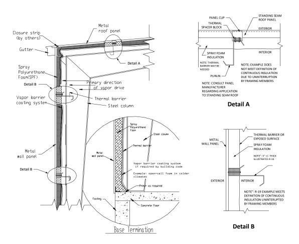
Figure 4 - Vapor Drive Toward Outside SPF Applied on Interior. Details A and B from Figures 5.2.11 and 5.2.14 in Metal Building Manufacturers Association (MBMA) document
