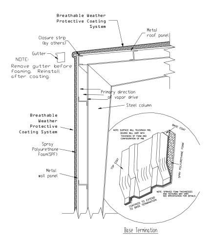
Figure 2 - Vapor Drive Toward Exterior, SPF Applied to Exterior
