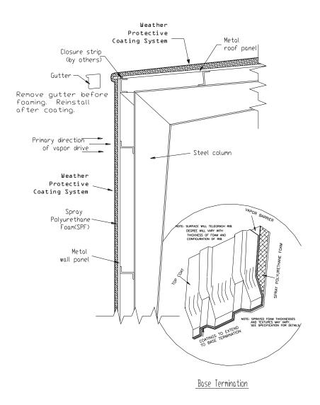
Figure 1 - Vapor Drive Toward Inside, SPF Applied to Exterior
