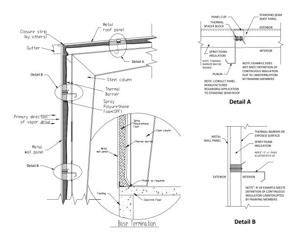
Figure 3 - Vapor Drive Toward Inside SPF Applied on Interior. Details A and B from Figures 5.2.11 and 5.2.14 in Metal Building Manufacturers Association (MBMA) document
