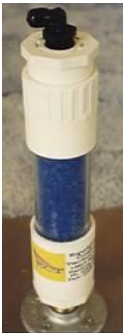
Figure 4 - Silica Gel Dryer mounted in ¾" hole of A-side Drum
