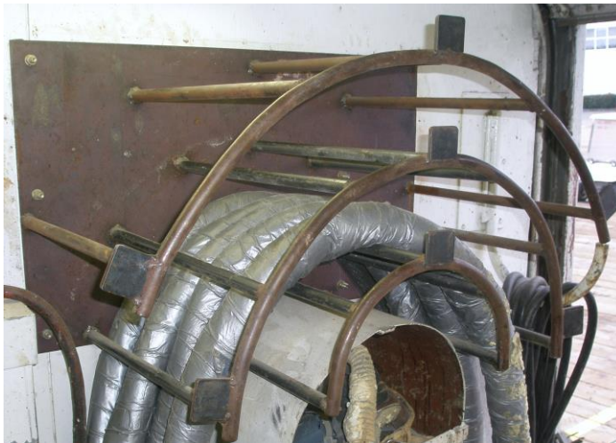
Figure 15 - Three-tiered rack hangs the hose in single layers, preventing electromagnetic effect and overheating of the hoses, enabling preheating of the entire hose while on the rack.
